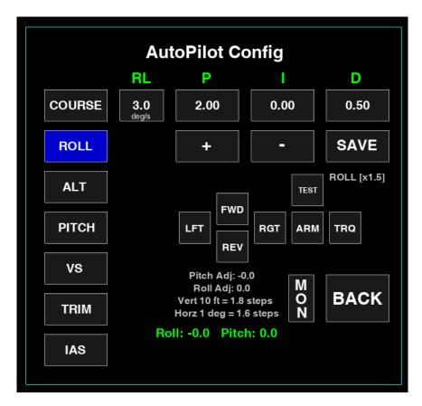
• When the autopilot is **active**, it opens the **Monitor Menu**, where real-time autopilot behavior can be observed and fine-tuned
