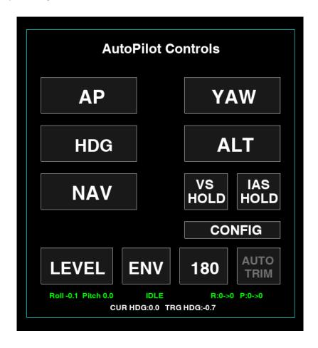
The AutoFlight menu interface provides access to all primary autopilot functions, including:
