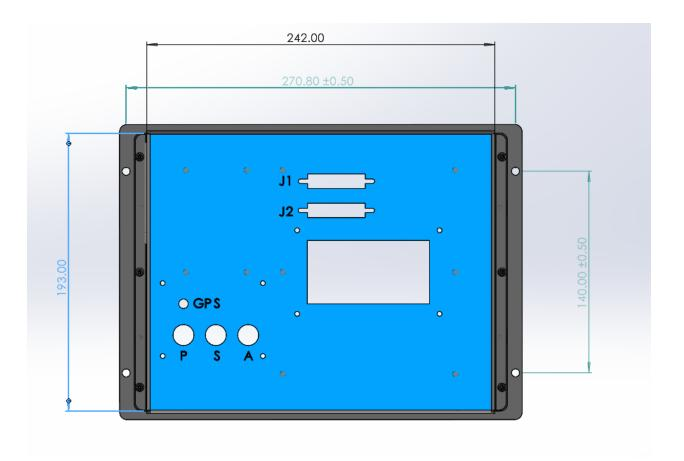
ELM1000 EFIS requires four (4) machine screws or bolts for panel installation. EFIS has four (4) holes in its front panel with a dimeter of 5.50mm each. It is recommended to use a mounting hardware of the size no less than #8-32
