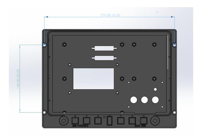
At the back side of the EFIS there are connectors so it is recommended to have a clearance with other parts of at least 120mm.
