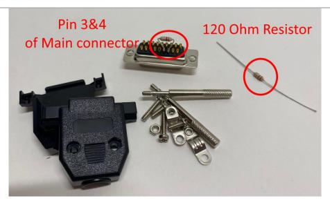
⚠ Important installation warning: Make sure that whenever VICS is installed and connected via CAN bus line to compatible EFIS module, the termination 120 Ohm resistor in EFIS's connector is removed while termination resistor at VICS connector is added. There must be only one termination resistor on the CAN bus at the very end of the CAN line.
