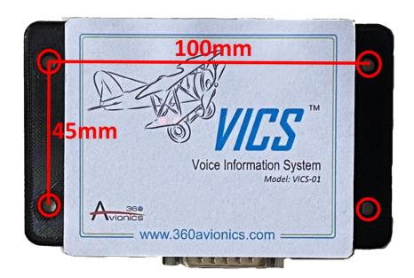
The installation depth of the VICS module will require approximately 125mm (including depth of the plugged D-SUB connector).
